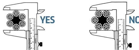
**Step 2:** Go to the shackles and confirm the stranding (6 or 8) of the ropes. Almost all compensating and governor ropes have 8 strands. Look at the rope tag to determine breaking load and then refer to the information in the Draka EHC catalog for the correct grade (Iron or Traction).
