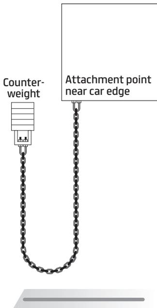
Compensating cable came about as a way to make chain quieter. Most compensating cables are some version of a coated chain and are about as flexible as chain. This was intentional; since compensation cable often replaced chain, it needed to form the same narrow loop as chain to connect to the same support points underneath the car and counterweight.
